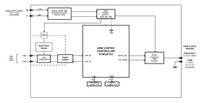
Figure 1 – Hardware Functional Block Diagram
