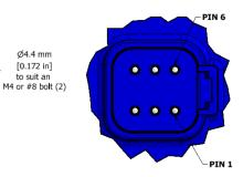
DETAIL A molded in Deutsch IPD DT04-6P receptacle <u>mates with</u>: Deutsch IPD DT06-6S
