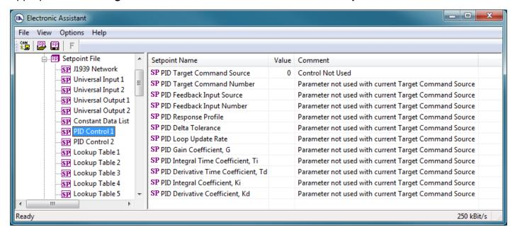
Figure 9 - Screen Capture of PID Control Setpoints
