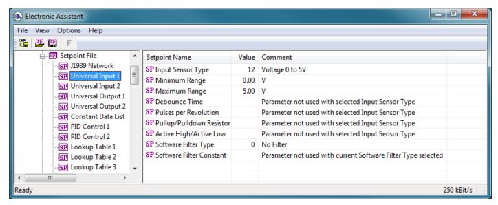
Figure 6 - Screen Capture of Universal Input Setpoints
