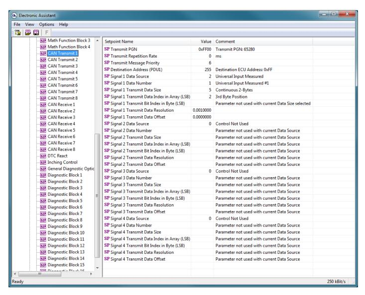
Figure 13 - Screen Capture of CAN Transmit Message Setpoints
