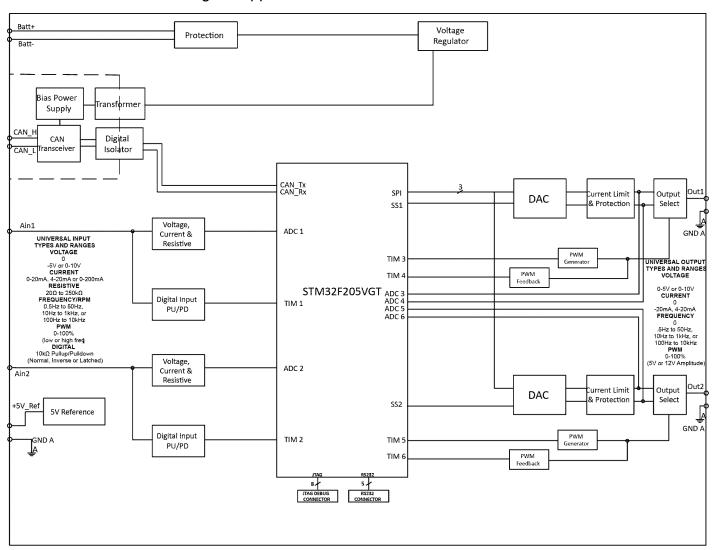
Figure 1 – Hardware Functional Block Diagram
