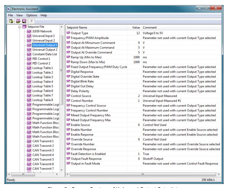
Figure 7 - Screen Capture of Universal Output Setpoints
