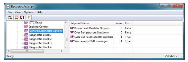
Figure 17 - Screen Capture of General Diagnostics Options Setpoints
