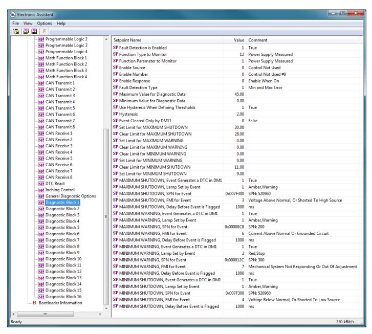
Figure 18 - Screen Capture of Diagnostic Block Setpoints
