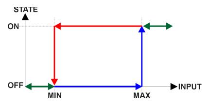
Figure 3 - Analog source to Digital input
