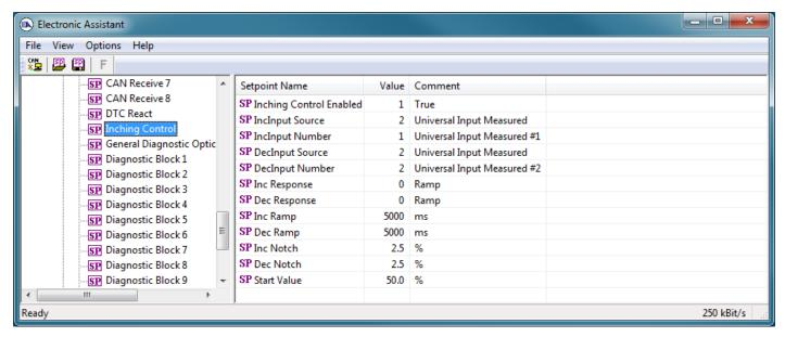
Figure 16 - Screen Capture of Inching Control Setpoints
