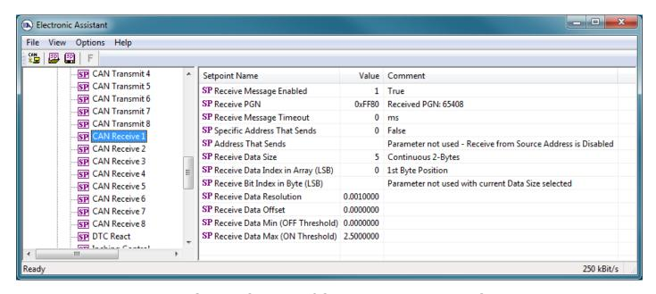
Figure 14 - Screen Capture of CAN Receive Message Setpoints
