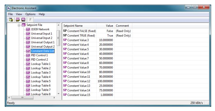
Figure 8 - Screen Capture of Constant Data List Setpoints
