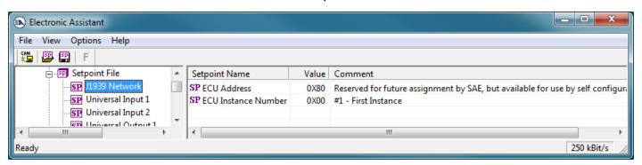
Figure 5 - Screen Capture of J1939 Setpoints
