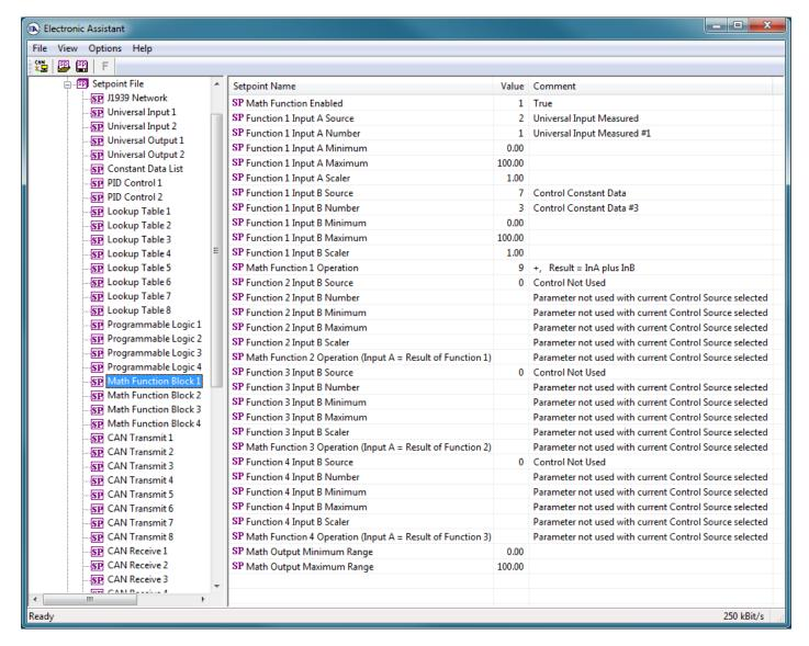
Figure 12 - Screen Capture of Math Function Block Setpoints
