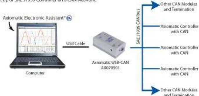
Set up of SAE J1939 Controller on a CAN Network:
