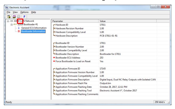
6. Select the <u>F</u>lashing button and navigate to where you had saved the **AF-17145\_x.yy.bin** file sent from Axiomatic. (Note: only binary (.bin) files can be flashed using the Axiomatic EA tool)
