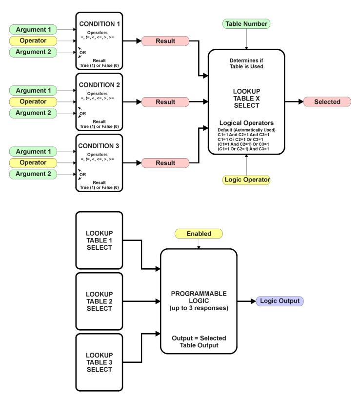
Figure 7: Programmable Logic Function Block
