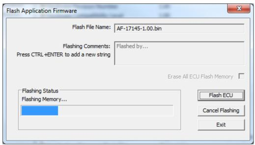
9. Once the firmware has finished uploading, a message will popup indicating the successful operation. If you select to reset the ECU, the new version of the AX031901 application will start running, and the ECU will be identified as such by the Axiomatic EA. Otherwise, thenext time the ECU is power-cycled, the AX031901 application will run rather than the bootloader function.
