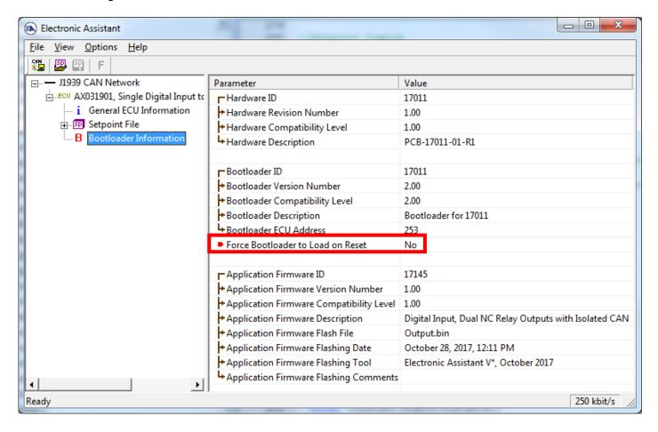
2. To use the bootloader to upgrade the firmware running on the ECU, change the variable "Force Bootloader To Load on Reset" to Yes.
