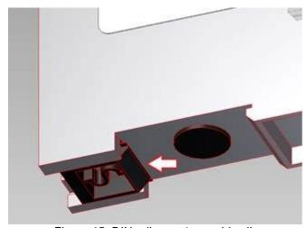
Figure 15: DIN rail mount movable clip
