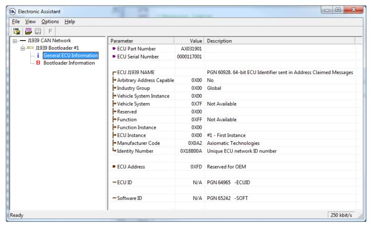
Note that the bootloader is NOT Arbitrary Address Capable. This means that if you want to have multiple bootloaders running simultaneously (not recommended) you would have to manually change the address for each one before activating the next, or there will be address conflicts, and only one ECU would show up as the bootloader. Once the 'active' bootloader returns to regular functionality, the other ECU(s) would have to be power cycled to re-activate the bootloader feature.
