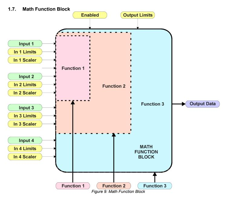
There are four mathematic function blocks that allow the user to define basic algorithms. A math function block can take up to four input signals, as listed in Table 19 in Section 1.12. Each input is then scaled according the associated limit and scaling setpoints.
