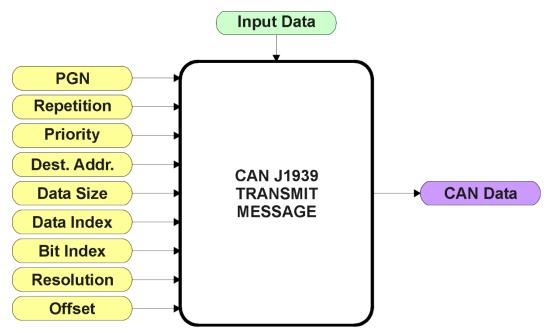
Figure 12: CAN Transmit Function Block
