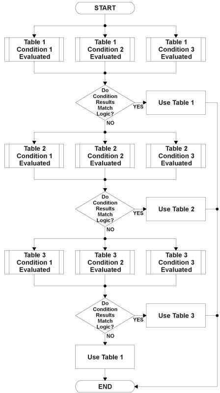
Figure 8: Programmable Logic Flowchart
