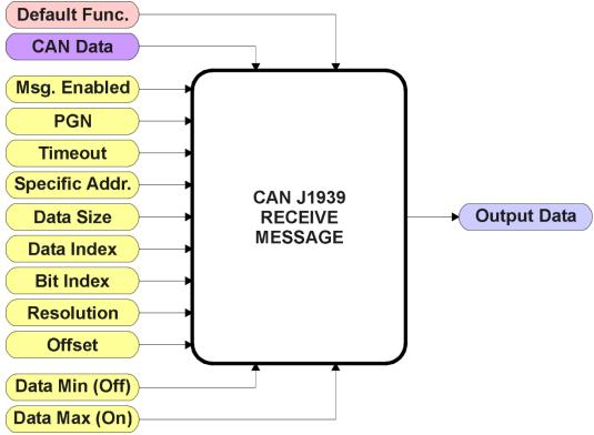
Figure 13: CAN Receive Function Block
