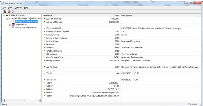
Note: The information provided in the Software ID is available for any J1939 service tool which supports the PGN -SOFT.
