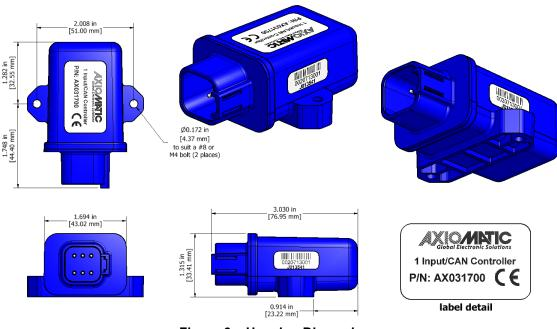
Figure 6 – Housing Dimensions
