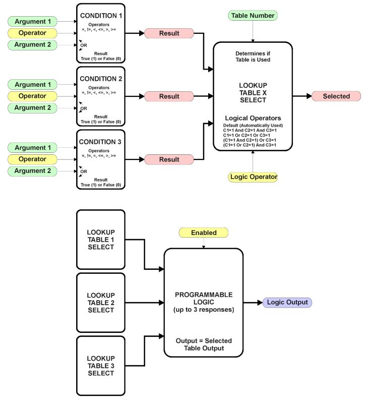
Figure 3 – Programmable Logic Function Block
