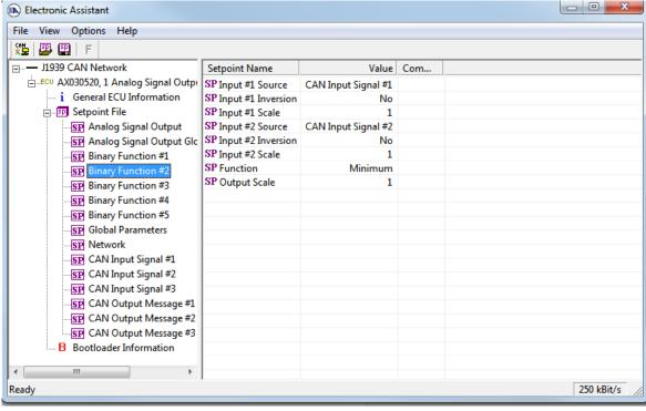
Then, calculate the displacement angle for positive and negative angle displacement using the Binary Function #2 and #3 function blocks:
