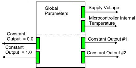
Two out of four constant logical outputs are user programmable. Other two represent logical one and logical zero outputs.
