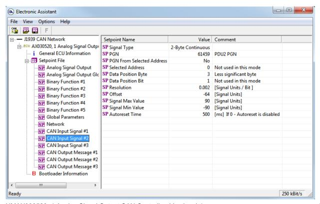
Now, when the data acquisition part of the pitch and roll CAN signals is set up, configure the data processing part of the controller to generate the displacement signal output.
