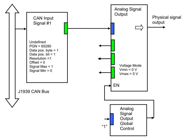
Unused function blocks and Global Parameters function block are not shown. The Analog Signal Output is at 0V independently of the CAN input signals. Uses can use this configuration as a template to build their own system configurations.
