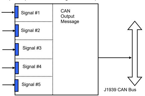
The CAN Output Message does not have a specific destination address. In case the message PGN is presented in the PDU1 format, the message is sent to the global address.
