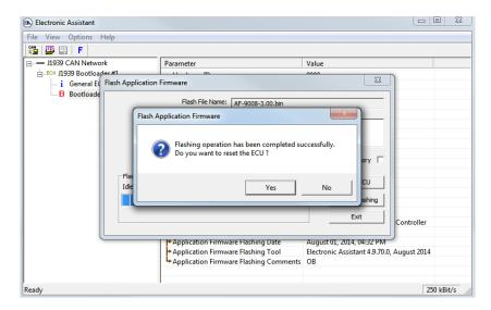
Select "Yes" and see the ECU running the new firmware. This will indicate that the flashing operation has been performed successfully.
