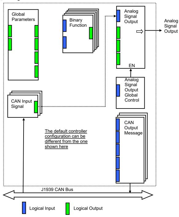
As an example, the logical output of the CAN Input Signal function block is connected to the logical input of the Analog Signal Output function block, providing a direct path for the CAN input signal to the controller signal output.
