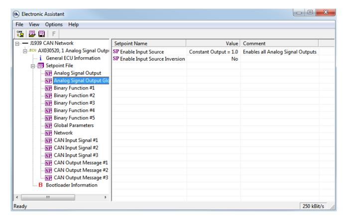
Then, configure the <u>Analog Signal Output</u> function block. Set the *Output Mode* setpoint to "Output Voltage", the *Vmin – Minimum Output Voltage* to 0V, and the *Vmax – Maximum Output Voltage* to +9V:
