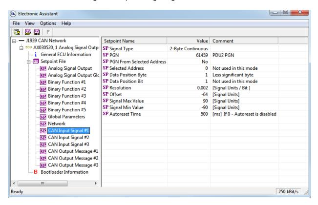
Similarly configure the <u>CAN Input Signal</u> #2 function block for receiving the roll angle signal:
