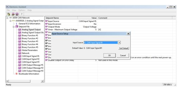
If the user changes the configuration parameter, the new value will be stored in a non-volatile memory and used immediately by the converter.
