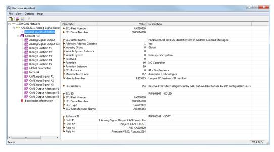
The configuration parameters are grouped by function blocks. Please, refer to the appropriate section of this manual describing the required function block.
