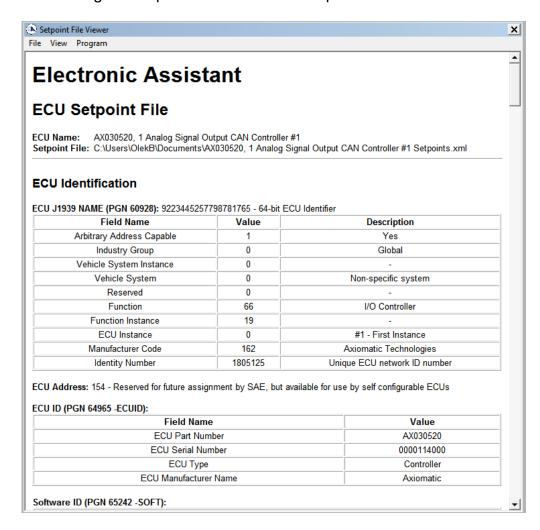
The CAN network identification and "read-only" configuration parameters are not transferrable using this operation. Also, the converter will perform one or several internal resets of all function blocks during the setpoint flashing operation.
