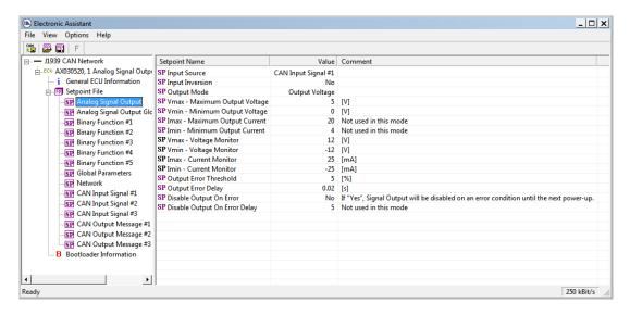
The user can view and, when necessary, change configuration parameters by double-clicking on the appropriate setpoint name. A pop-up dialog window will appear:
