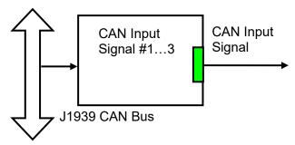
The <u>CAN Input Signal</u> function block has an ability to filter out signals transmitted only from a selected address. This way, it can be bound to a specific ECU on the CAN network. It can also automatically reset the input signal data in case the signal has been absent or lost for more than a specific period of time.
