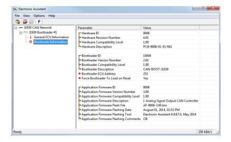
At this point, the user can return to the installed controller firmware by changing the *Force Bootloader to Load on Reset* flag back to "No" and resetting the ECU.
