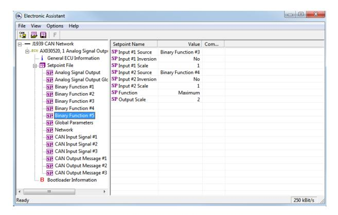
The calculated displacement angle value will go directly to the <u>Analog Signal Output</u> function block, as it has already been configured in <u>Analog Signal Output</u>.
