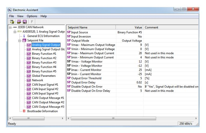
Now, configure the <u>CAN Input Signal</u> #1 and <u>CAN Input Signal</u> #2 function blocks to accept pitch and roll signals from the CAN bus. According to the J1939/71 standard, these signals are transmitted in PGN 61459 (Slope Sensor Information) as SPN 3318 (Pitch Angle) and SPN 3319 (Roll Angle), see the following table:
