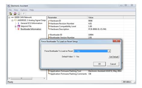
The Axiomatic EA will prompt the user to change the *Force Bootloader to Load on Reset* parameter flag to "Yes". This will automatically activate the bootloader on the next ECU reset. After accepting the change, the next screen will ask the user if the reset is actually required. Select "Yes".
