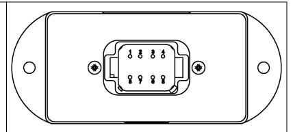
8-pin plug (equivalent TE Deutsch P/N: DT15-08PA)
