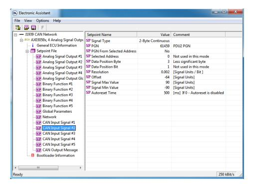
Now, when the pitch and roll analog output signals are set up, configure the emergency signal output.
