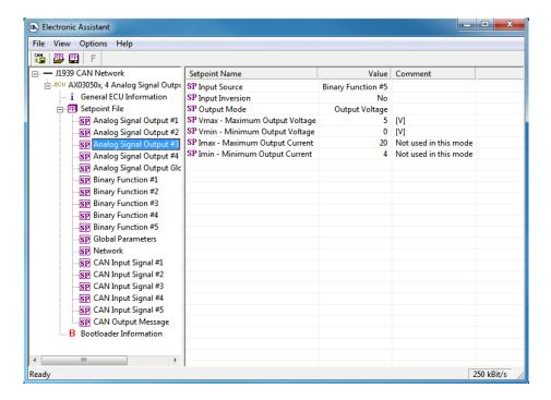
The controller setpoints are now programmed. The user can save the controller setpoint configuration into a setpoint file for the future reference or for programming of the other controllers.
