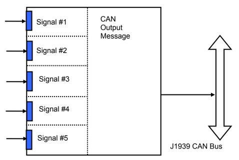
The message does not have a specific destination address. In case the PGN of the message is presented in the PDU1 format, the message is sent to the global address.
