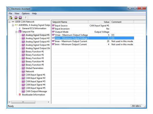
Do the same manipulations with the <u>Analog Signal Output</u> #2 function block, with an exception of connecting its logical input to the logical output of the <u>CAN Input Signal</u> #2 function block.
