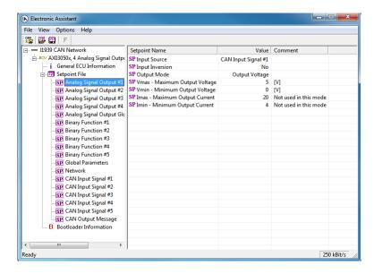
The user can view and, when necessary, change setpoints by double-clicking on the appropriate setpoint name. The setpoint pop-up dialog window will appear:
