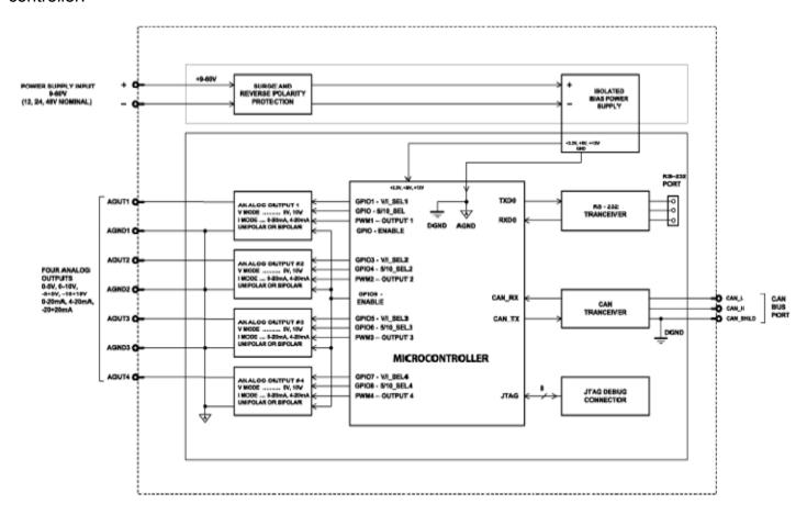
Figure 1. The Controller Hardware Block Diagram.
