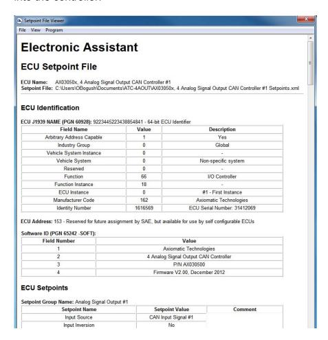
The network identification and "read-only" setpoints are not transferrable using this operation. Also, the controller will perform one or several internal resets of all function blocks during the setpoint flashing operation.
