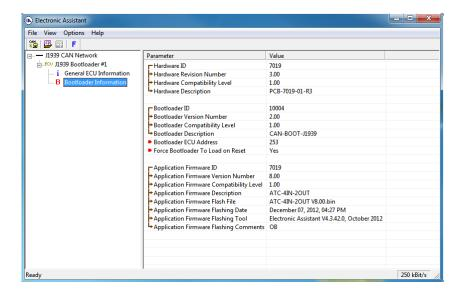
At this point, the user can return to the installed controller firmware by changing the *Force Bootloader to Load on Reset* flag back to *No* and resetting the ECU.
