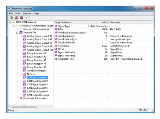
Similarly configure the <u>CAN Input Signal</u> #2 function block for receiving the roll angle signal.
