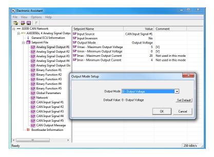
The controller will perform an internal reset of all function blocks after each change of the setpoints. If the new setpoint affects the network identification, the controller will reclaim its network address with a new network identification message, see <u>J1939 Name and Address</u>.
