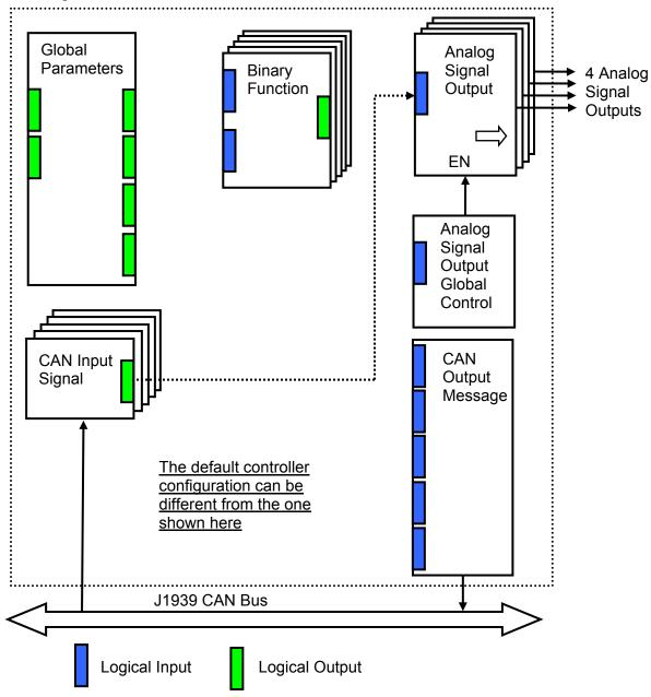
As an example, the logical output of the CAN Input Signal function block is connected to the logical input of the Analog Signal Output function block, providing a direct path for the CAN input signal to the controller signal output.
