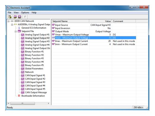
Now, configure the <u>CAN Input Signal</u> #1 and <u>CAN Input Signal</u> #2 function blocks to accept pitch and roll signals from the CAN bus. According to the J1939/71 standard, these signals are transmitted in PGN 61459 (Slope Sensor Information) as SPN 3318 (Pitch Angle) and SPN 3319 (Roll Angle), see the following table:
