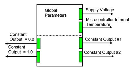
Two out of four constant logical outputs are user programmable. Other two represent logical one and logical zero outputs.
