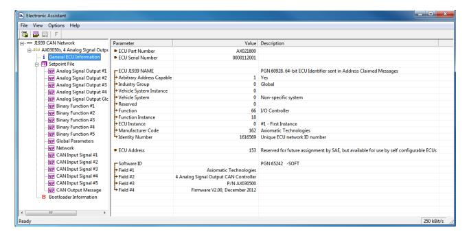
The setpoints are grouped on the base of their functionality. Please, refer to the appropriate sections of this manual describing the required function block or a setpoint group.
