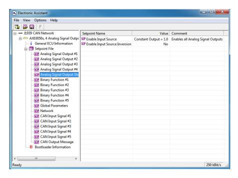
Then, program with the <u>Analog Signal Output</u> #1 function block. Set the *Output Mode* setpoint to "Output Voltage", the *Vmax – Maximum Output Voltage* to +5V, and the *Vmin – Minimum Output Voltage* to -5V. Also, connect the logical input of this function block to the logical output of the <u>CAN Input Signal</u> #1 function block using the *Input Source* setpoint. Finally, ensure that you do not invert the logical input data and the *Input Inversion* setpoint is set to "No".
