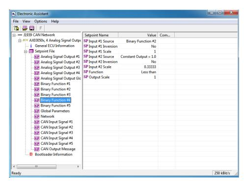
Now use <u>Binary Function</u> #5 function block to combine minimum and maximum "out of range" conditions into one signal using the logical OR function.
