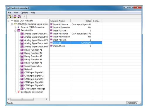
Then, configure <u>Binary Function</u> #3 and #4 function blocks to detect conditions when the minimum and maximum angles go out of range. Use Constant Output = 1.0 logical output together with the input scale setpoints to create appropriate thresholds.
