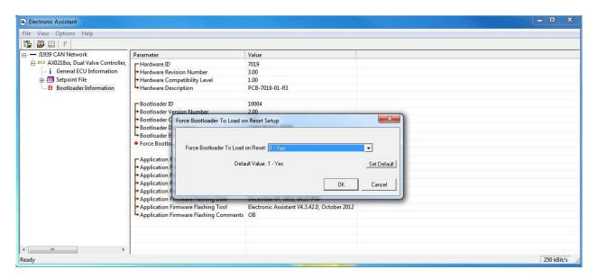
The EA will prompt the user to change the *Force Bootloader to Load on Reset* parameter flag to Yes. This will automatically activate the bootloader on the next ECU reset. After accepting the change, the next screen will ask the user if the reset is actually required. Select Yes.
