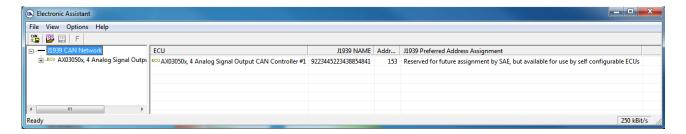
For 500kBit/s and 1Mbit/s controllers the baud rate in the bottom-right part of the screen will be different.
