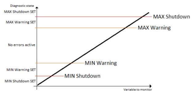
Figure 3 – Double Minimum and Maximum Error Thresholds
