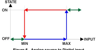
Figure 6 - Analog source to Digital input
