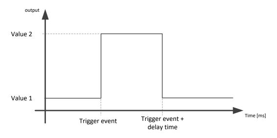
Figure 4 – Delay Timer output vs Time
