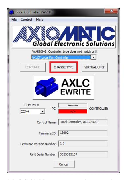
The last button, *VIRTUAL UNIT* allows you to go to select any model type, and see the corresponding configuration screen without having an actual unit connected. This is a helpful feature when you want to create, review or edit a configuration file (.vdr, .fdr or .tdr), or to demonstrate the features of the programming tool. When a *VIRTUAL UNIT* has been selected, the Read and Write buttons are disabled for all types of controllers.
