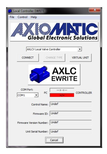
Before connecting to the unit, make sure that the appropriate COM port has been selected for your computer. By default, the program will use COM1, but you can select a different port if necessary.
