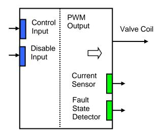
The user can select: the output mode, minimum and maximum output values, dither parameters, and ramps. Also, PID coefficients can be set to control the output current in the "Output Current" mode. For the current sensor, the user can define an averaging time to minimize effect of the output dither on the sensor readings.
