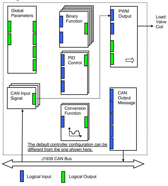
As an example, the logical output of the CAN Input Signal functional block is connected to the logical input of the PWM Output functional block, providing a direct path for the CAN input signal to the controller output.
