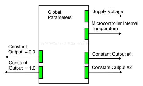
Two out of four constant logical outputs are user programmable. Other two represent logical one and logical zero outputs.
