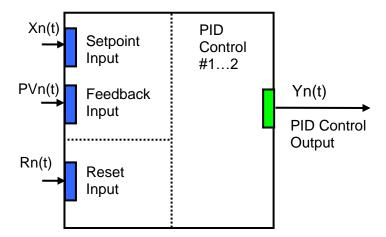
The normalized output of the <u>PID Control</u> functional block Yn(t), as a function of time, can be described by the following formula:
