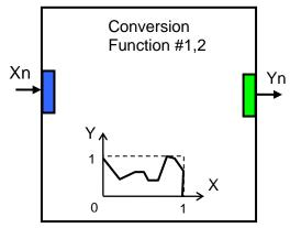
The function F(x) is defined using a piecewise linear approximation in up to 11 points. Each point is presented by three parameters:
