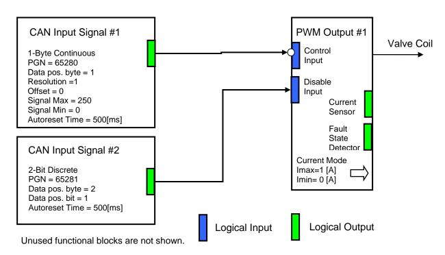
Figure 3. The Block Diagram of the Controller Configuration for the Setpoint Programming Example.
