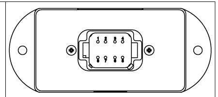
8-pin plug (equivalent TE Deutsch P/N: DT15-8PA)
