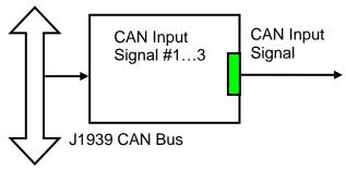
The <u>CAN Input Signal</u> functional block has an ability to filter out signals transmitted only from a selected address. This way, it can be bound to a specific ECU on the CAN network. It can also automatically reset the input signal data in case the signal has been absent or lost for more than a specific period of time.
