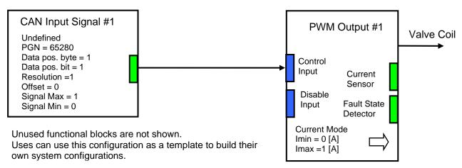
Figure 2. The Block Diagram of the Default Controller Configuration
