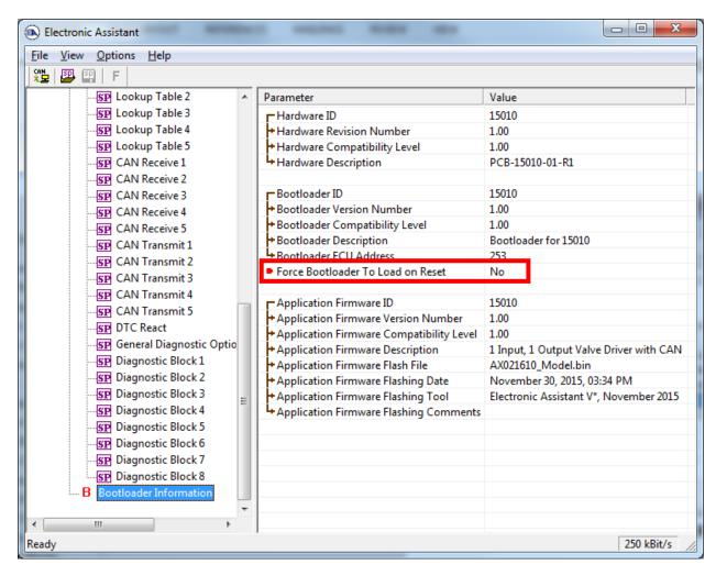
2. To use the bootloader to upgrade the firmware running on the ECU, change the variable "Force Bootloader To Load on Reset" to Yes.
