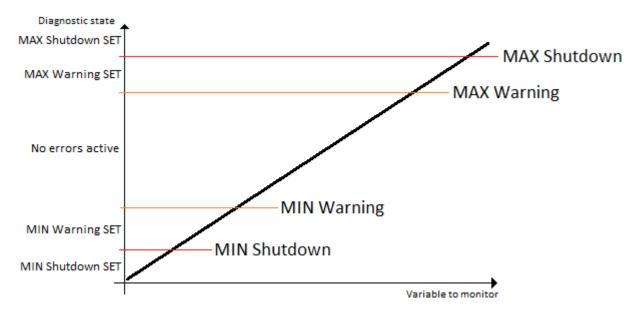
Figure 4 – Double Minimum and Maximum Error Thresholds
