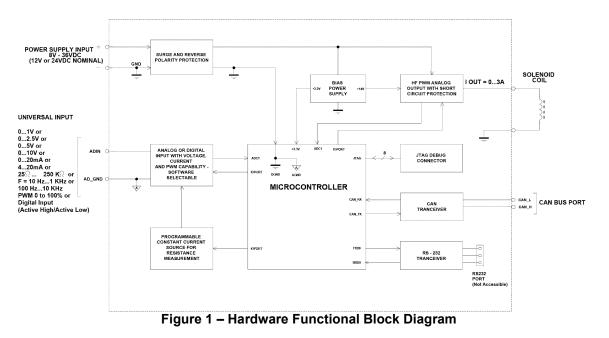
The controller (1IN-1OUT-LED) is designed for versatile control of a universal input and a proportional valve output. Its flexible hardware design allows for the controller to have a wide range of input and output types. The sophisticated control algorithms/logical function blocks allow the user to configure the controller for a wide range of applications without the need for custom firmware.
