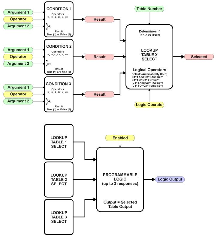
Figure 7 – Programmable Logic Function Block
