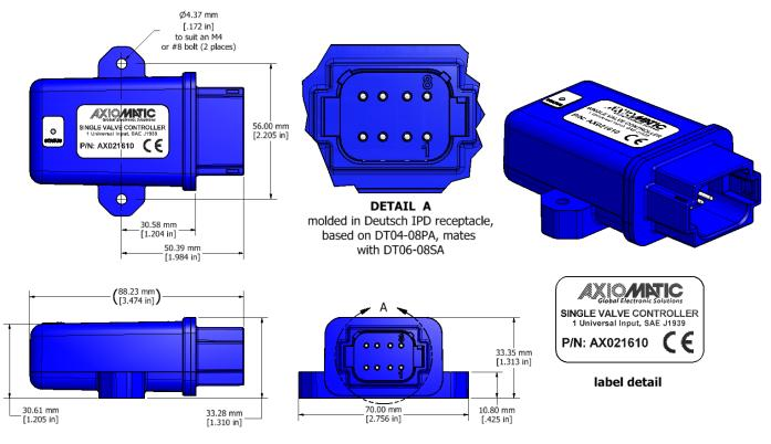
Figure 9 – Housing Dimensions
