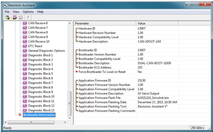
2. To use the bootloader for upgrading the firmware running on the ECU, change the variable "Force Bootloader To Load on Reset" to Yes.
