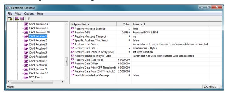
Figure 15 - Screen Capture of CAN Receive Message Setpoints
