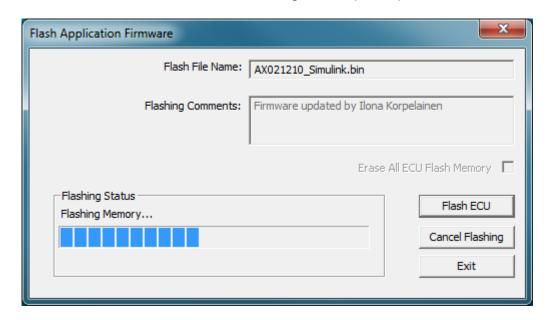
Once the firmware has finished uploading, a message will pop up indicating the successful operation. If you select to reset the ECU, the new version of the AX021210 application will start
