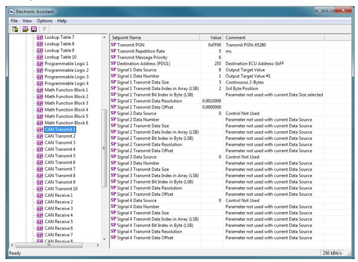
Figure 14 - Screen Capture of CAN Transmit Message Setpoints
