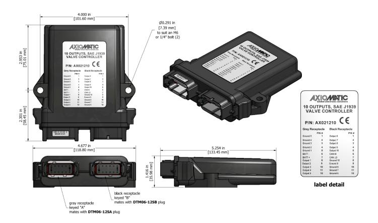
Figure 5 - AX021210 Dimensional Drawing
