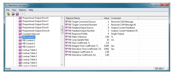
Figure 10 - Screen Capture of PID Control Setpoints
