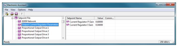
Figure 7- Screen Capture of Output Current Regulator Parameters Setpoints
