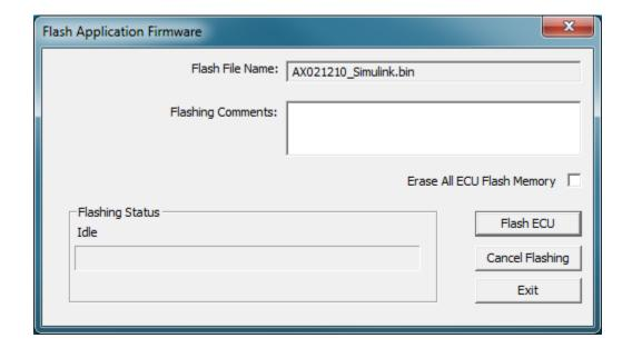
WARNING: Do not check the "Erase All ECU Flash Memory" box unless instructed to do so by your Axiomatic contact. Selecting this will erase ALL data stored in non-volatile flash including the calibration from Axiomatic factory testing. It will also erase any configuration of the setpoints that might have been done to the ECU and reset all setpoints to their factory defaults. By leaving this box unchecked, none of the setpoints will be changed when the new firmware is uploaded.
