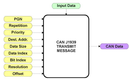
Figure 21 – CAN Transmit Function Block
