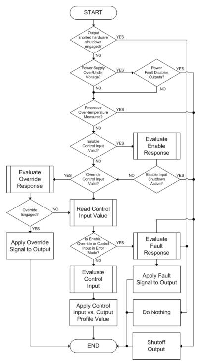
Figure 4 – Output Logic Flowchart
