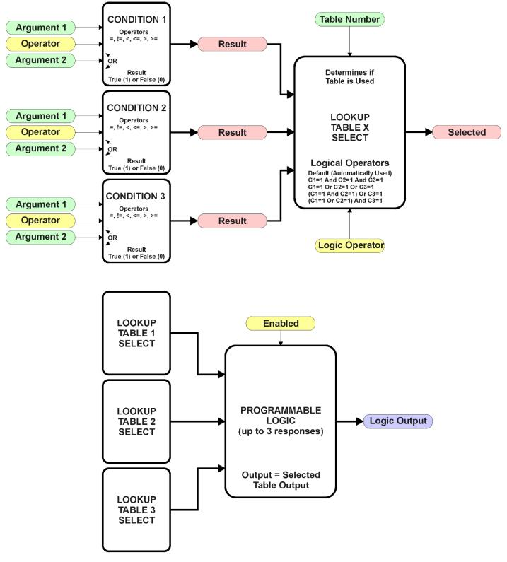
Figure 16 – Programmable Logic Function Block
