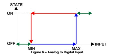
If a digital **"Output Type"** has been selected, the **"Digital Response"** setpoint will be enabled as shown in Table 4. Also, the **"Digital Override State"** setpoint will be enabled, and will follow the Override input the same way that the **"Output at Override Command"** would be used with a proportional output response.
