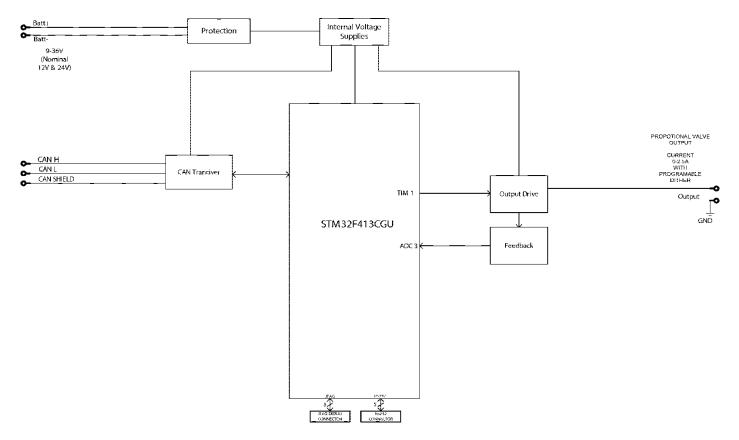
Figure 1 – Hardware Functional Block Diagram
