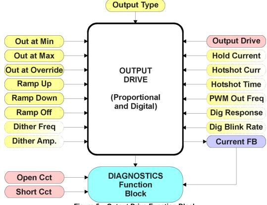
Figure 5 – Output Drive Function Block
