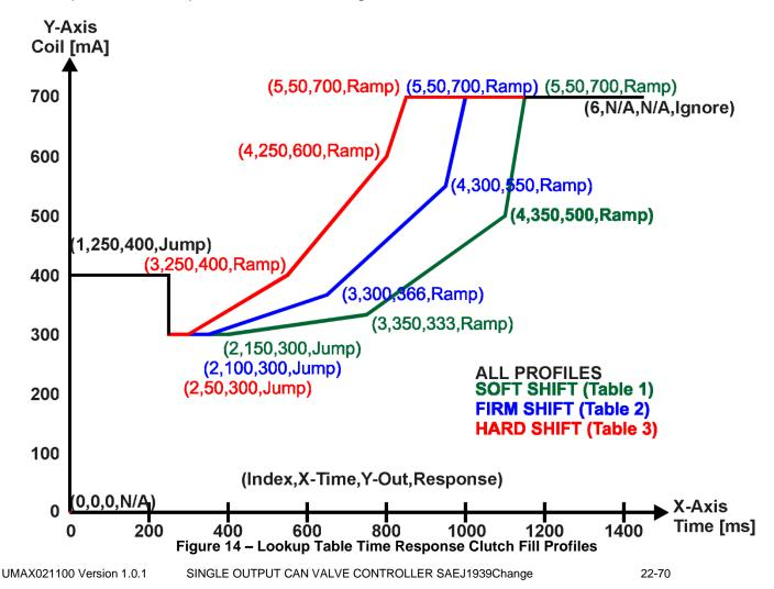
In a time response, the interval time between each point on the X-axis can be set anywhere from 1ms to 24 hours. [86,400,000 ms]
