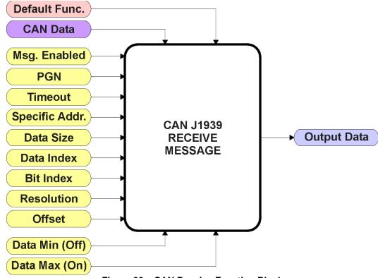
Figure 22 – CAN Receive Function Block
