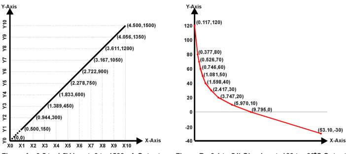
Figure A - 0.5 to 4.5V Input, 0 to 1500mA Output Figure B - 0.1 to 54kOhm Input, 120 to -30°C Output Figure 11 – Lookup Table Initialization Examples
