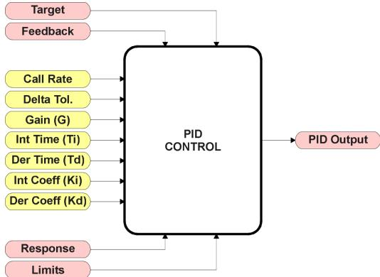
Figure 8 – PID Control Function Block
