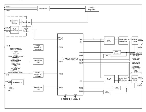
The controller belongs to a family of Axiomatic smart controllers with programmable internal architecture. This provides users with flexibility, allowing them to build a custom controller with their own required functionality from a set of predefined internal functional blocks using the PC-based Axiomatic Electronic Assistant software tool. Application programming is performed through the CAN interface, without disconnecting the controller from the user's system.
