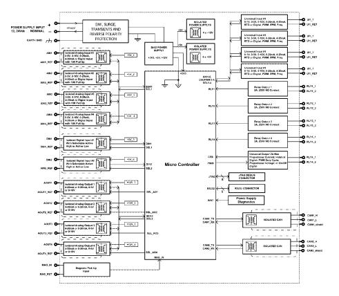
The controller belongs to a family of Axiomatic smart controllers with configurable internal architecture. This provides users with flexibility, allowing them to build their own custom controller with a required functionality from a set of predefined internal functional blocks using the commercially available software tools. Application programming is performed through the CAN interface, without disconnecting the controller from the user's system.
