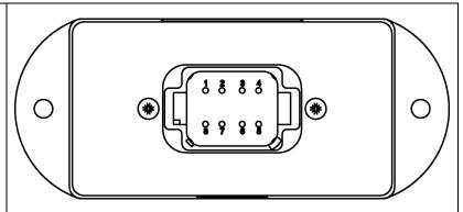
8-pin plug (equivalent TE Deutsch P/N: DT15-08PA)
