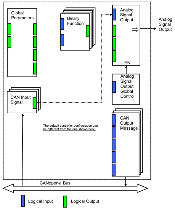
As an example, the logical output of the CAN Input Signal functional block is connected to the logical input of the Analog Signal Output functional block, providing a direct path for the CAN input signal to the controller signal output.
