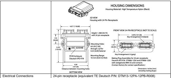
24-pin receptacle (equivalent TE Deutsch P/N: DTM13-12PA-12PB-R008) Mating plug: equivalent to the TE Deutsch P/Ns: DTM06-12SA and DTM06-12SB, with 2 wedgelocks (WM12S) and 24 contacts (0462-201-20141).
