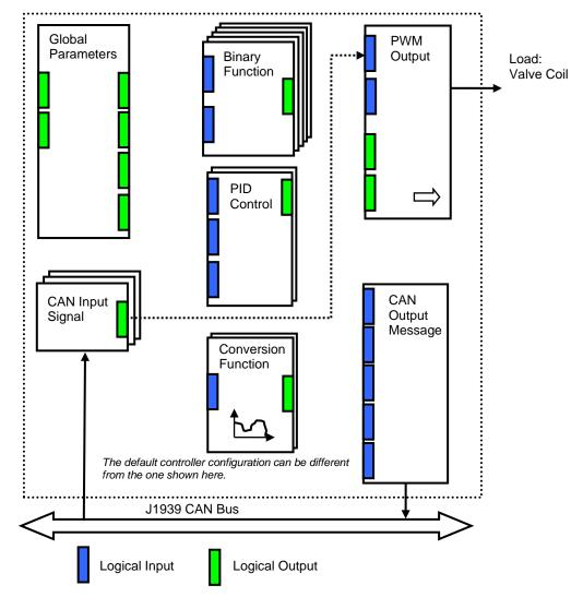
As an example, the logical output of the CAN Input Signal functional block is connected to the logical input of the PWM Output functional block, providing a direct path for the CAN input signal to the controller output.
