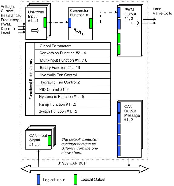
As an example, the Universal Inputs #1 functional block is connected to the Conversion Function #1 and the Conversion Function #1 is connected to the PWM Output #1 functional block, providing a path for the input signal from input to output through the Conversion Function #1 functional block.
