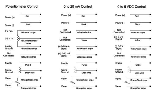
Refer to page 2 (block diagram) for an alternative method of connecting a current loop transmitter to provide a current control signal input. In this method, the current loop transmitter receives power from the power supply powering the amplifier. The transmitter is connected to the driver's +power supply input wire and the +0 to 20 mA input wire. This method does not use the -0 to 20 mA signal wire connection.
