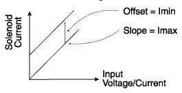
Adjusting the maximum current (I-max.) does not affect the minimum current (I-min.) setting.
