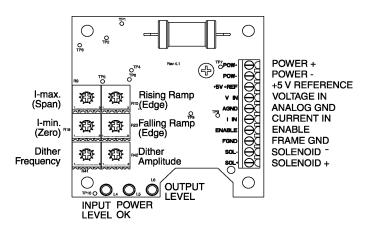
In the Metal Box Driver, adjustments are accessible by loosening the four screws on the lid of the housing and removing the lid.
